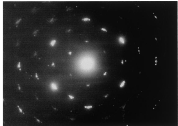
Figure 9 Electron diffraction pattern of the matrix composed by crystallites after deformation. The set of concentric hexagonal diffraction rings is typical for ultra-fine crystalline material characterised by a preferred crystallographic orientation.
